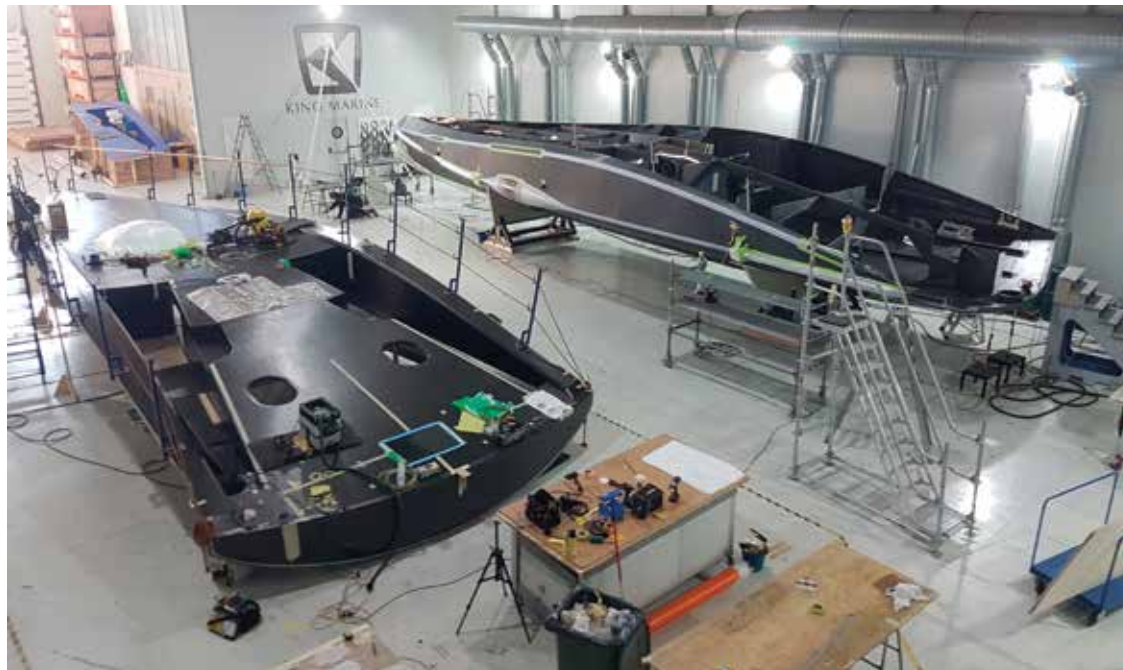
Significant moment in the construction at King Marine, when FlyingNikka 's hull and deck were united.
